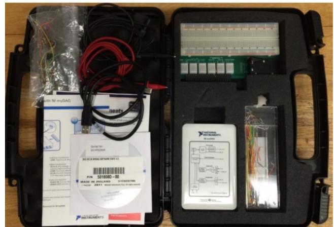
*Fig.1 Interior of NI DAQ kit*
